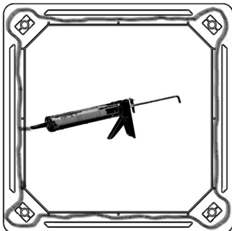
Figure 5 - Recommended sealant path
