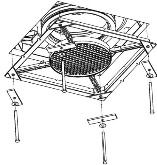
Figure 9- Assemble Bolt, washer & bar into duct & brace
